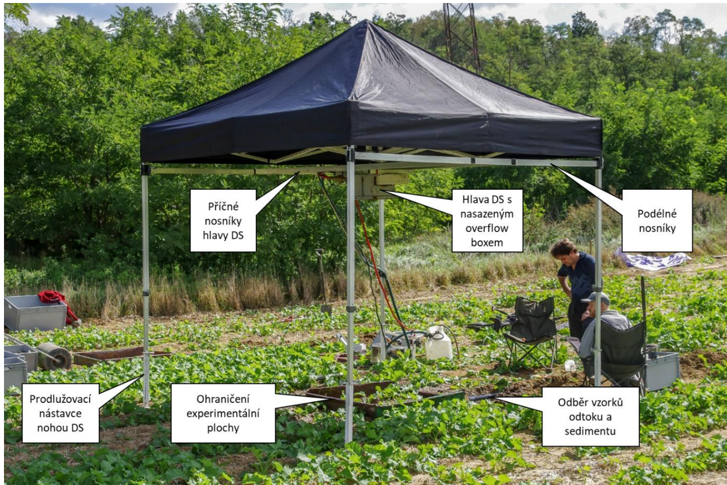
Mobile (small) rainfall simulator with variable rainfall intensities
