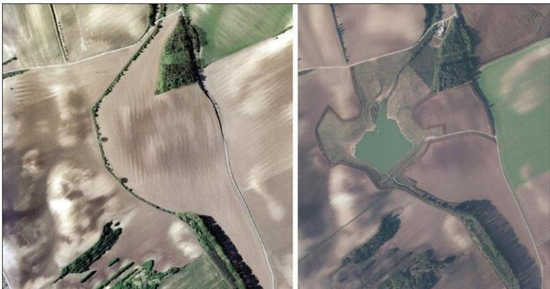
Situation before and after the design of the protective water reservoir on the Šardický stream – total volume of the water reservoir 182 000 m<sup>3</sup>
