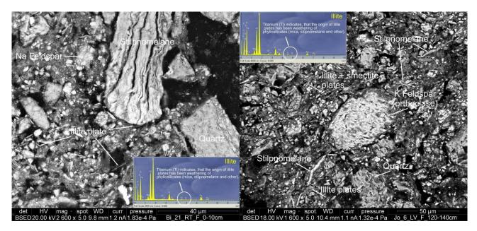
Fig. 4a. Clay minerals formed in weathered phyllosilicates (mica, stilpnomelane and others) in the soil of the Upper Pleistocene deposits (Western Lithuania, Bijotai)
