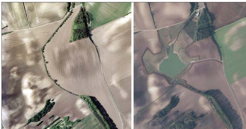
Situation before and after the design of the protective water reservoir on the Šardický stream – total volume of the water reservoir 182 000 m 3
