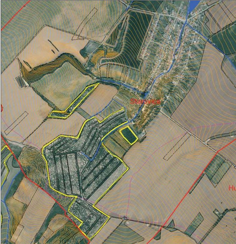
Figure 2. Bench terraces as an important flood protection measures
